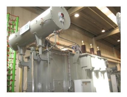
Three-Phase Oil Immersed Furnace Transformer for EAF Furnace Make "TES" (Transformer Electro Service) – nowadays "TAMINI"
